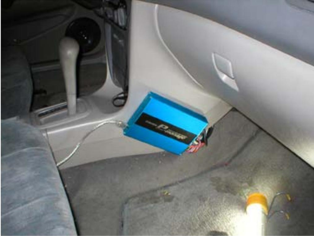
This eManage was mounted to the side of the console, however in your installation you can install it somewhere less visible. This one was mounted on the side for ease of access during the Spool Turbo kit installation for the 98-2002 Toyota Corollas.
