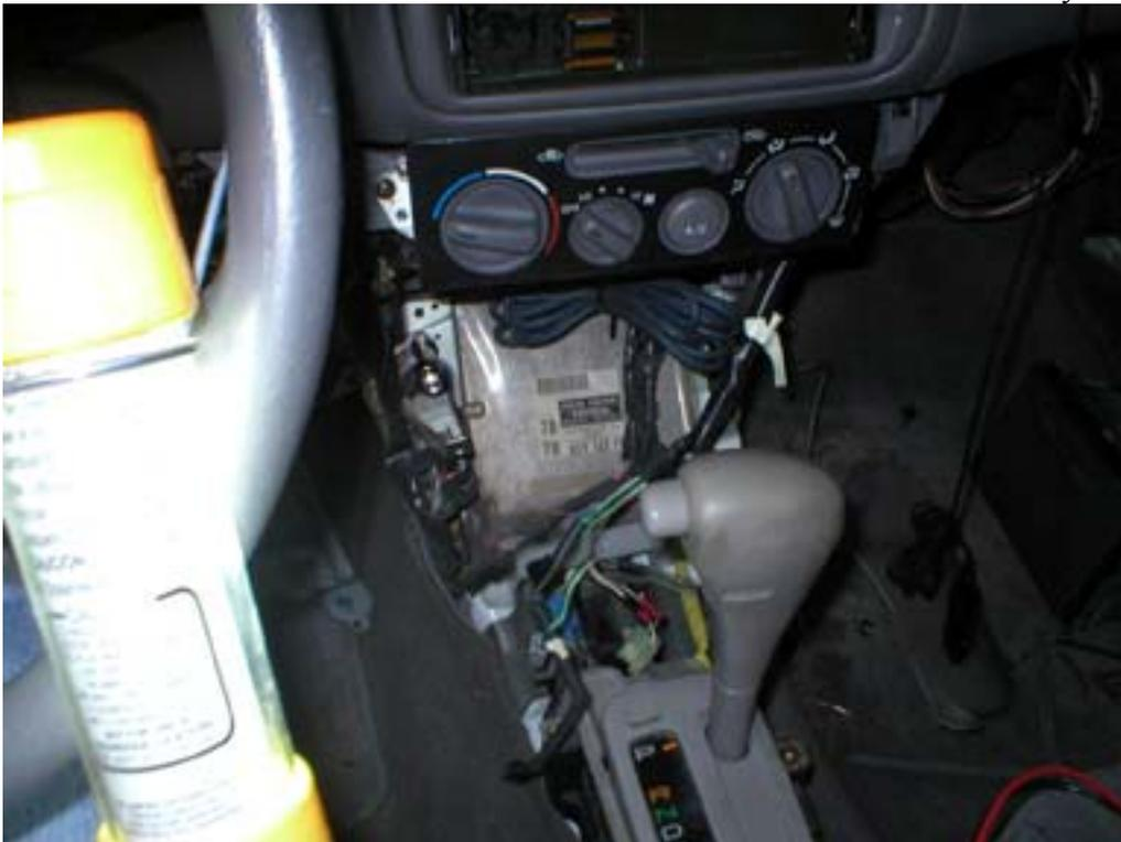
Once all the screws from the panels on either side of the console and the console itself are removed, you'll find the ECU sitting right there with three screws holding it mounting brackets in. Also when removing the console, note there are two screws inside the rear storage compartment under the bottom cover within it.
